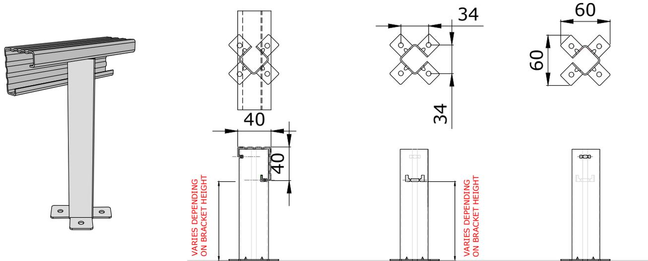
Brackets less than 260mm require 2 fixings diagonally opposite.
